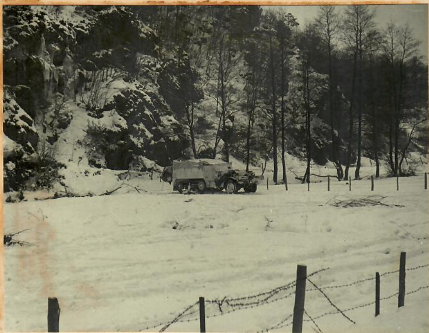
SNOW CAMOUFLAGE - Trucks, Reconnaissance Vehicles and Tanks were whitewashed to blend with snow backgrounds.
