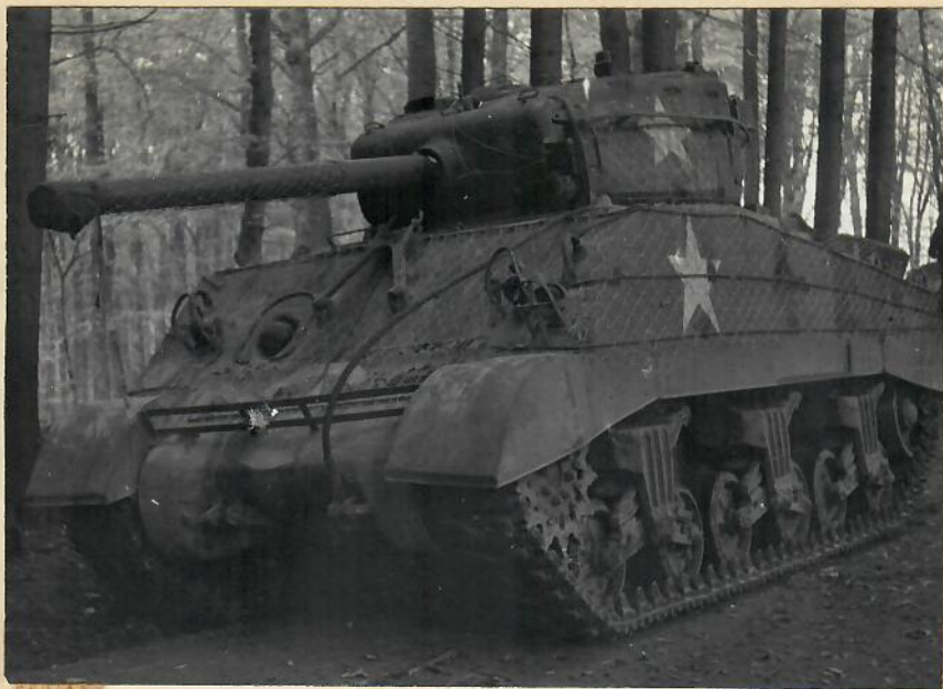
Sommerfeld mat applied to a tank, after which pattern painting is applied. Assistance and supervision of the work was provided by Cos B and D of the Bn.
