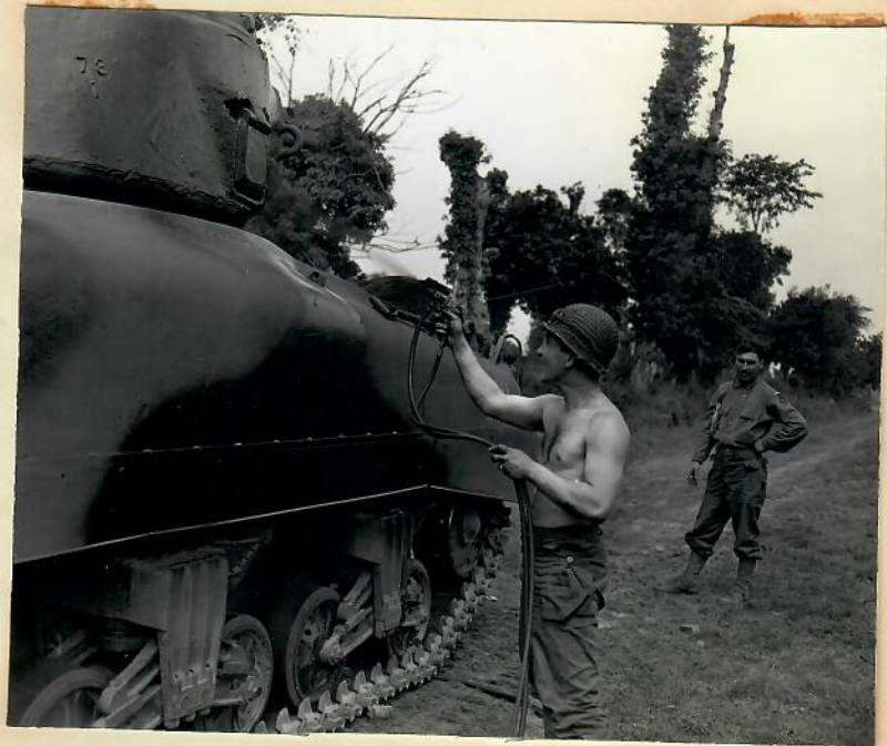
Pattern painting a tank. After the OD is applied over entire tank, black is sprayed on in large ir- regular pattern.
