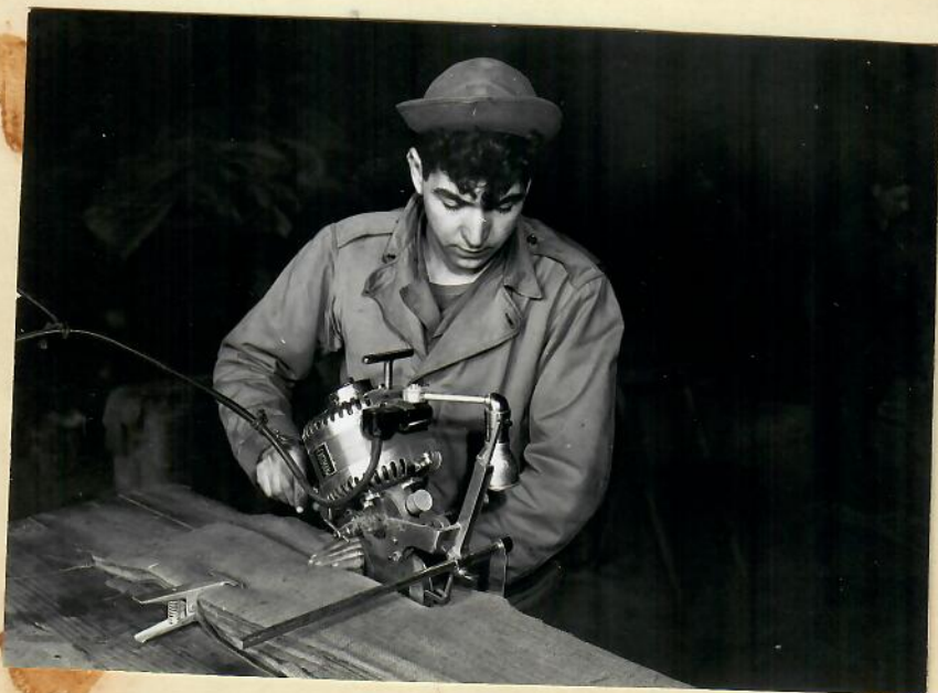
One of the few pieces of T&E equipment used in the manufacture of garlands. A rotary knife cutting the dyed and folded burlap into 2 inch widths.
