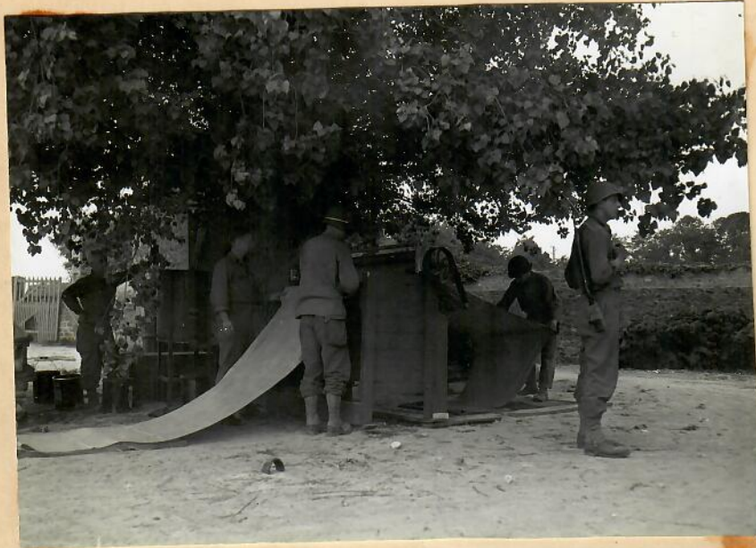
Home made electrically operated dipping vat for coloring undyed burlap
